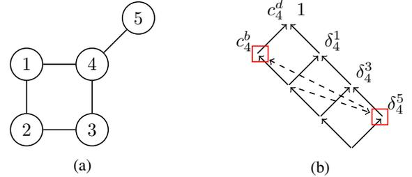
Fig. 3: Interconnection graph (a) and cost saving graph (b) of nCDN 4 in Example 1. The squares show the cost savings of nCDN 4 in the content allocation  $(a, b, c, d, d)$ .
